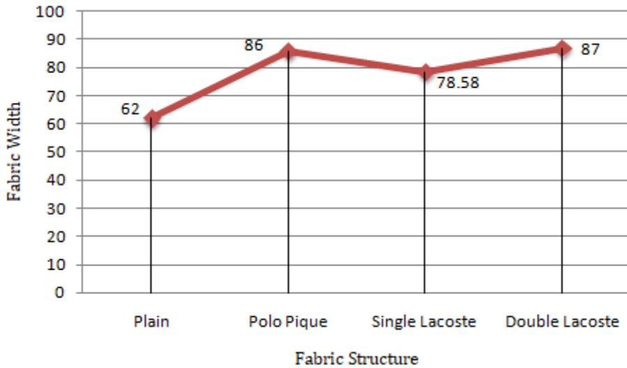
*Figure-1: Behavior of fabric width in different fabric structure*
