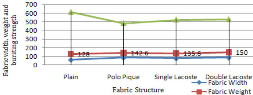
Figure-4: Behavior of fabric bursting strength, fabric weight and fabric width in different fabric structure
