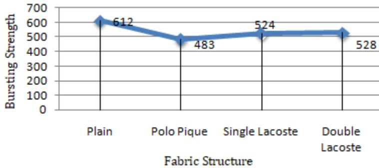
Figure-3: Behavior of fabric bursting strength in different fabric structure
